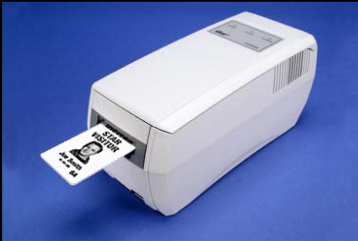
The TCP400 Thermal Card Printer/Re-Writer products offer the latest in thermal card technology, coupled with 3-track magnetic stripe read/write capability. The TCP400 can write an image to the “human-readable” area of the thermal media at 203 dpi or resolution and re-write that media up to 500 times.
