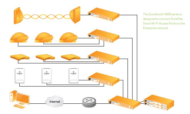
The ZoneSwitch 4000 supports up to 256 VLANs and dynamic VLANs with GVRP for separating type of traffic for seamless mobility.
