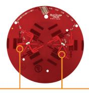
The high-gain directional antenna system specifically designed for spatial multiplexing, a technique used by 802.11n, provides multiple antenna elements that are controlled by an expert software system. This system determines the best antenna pair for any packet at any given time
