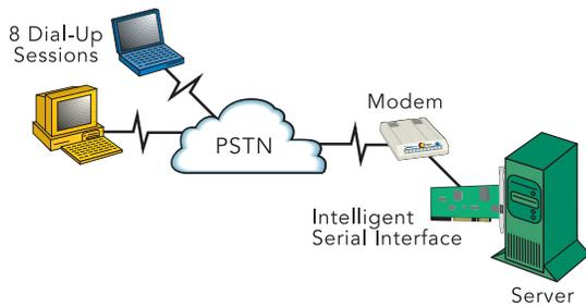
**Optimize System Performance.** The ISI processor off-loads the host CPU of communication functions providing optimum performance and preventing bottlenecks. And since all ports share the same IRQ, the server is not overloaded with IRQ assignments for the ISI card.
