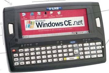
Large 6.5" high visibility mono or color display with touch screen for crystal-clear viewing.
