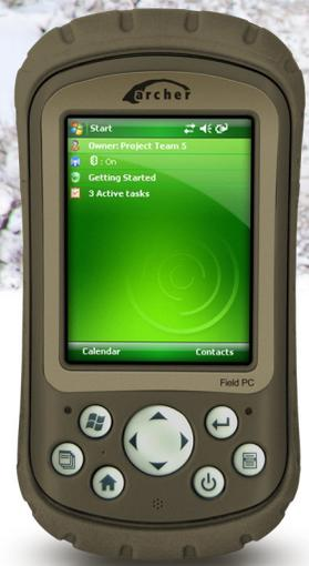
**Tested to MIL-STD-810F for water, humidity, sand and dust, vibration, altitude, shock, and temperature**
