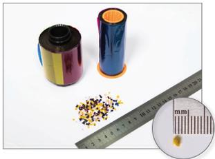
With the IDP's Twisted Micro-Cut Technology, SMART-BIT uses its unique twist and cut motions to completely shred ribbon panels into tiny particles. (\*Patent pending)
