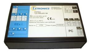
Galvanic isolation for keyboards, pointing devices, barcode scanners and other RS232/RS485 serial interfaces
