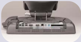
Bottom view, showing connectivity
