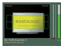
The second configuration step consists in setting the functioning parameters of the control previously selected and the acceptance thresholds.
