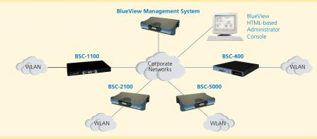
The BlueView™ Management System eliminates the labor-intensive task of configuring multiple devices deployed in multiple locations by enabling you to provision, configure, and manage all of your WLAN deployments remotely from a central location.
