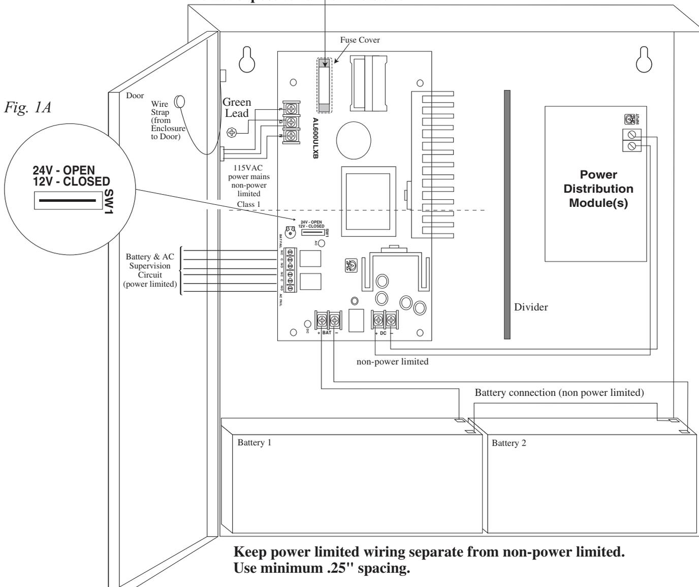
3. Secure cabinet to earth ground. Connect AC power (115VAC / 60 Hz to terminals marked [L, G, N] (*Fig. 1, pg. 3*). Use 14 AWG or larger for all power connections (Battery, DC output, AC input). Use 22 AWG to 18 AWG for power limited circuits (AC Fail/Low Battery reporting).
