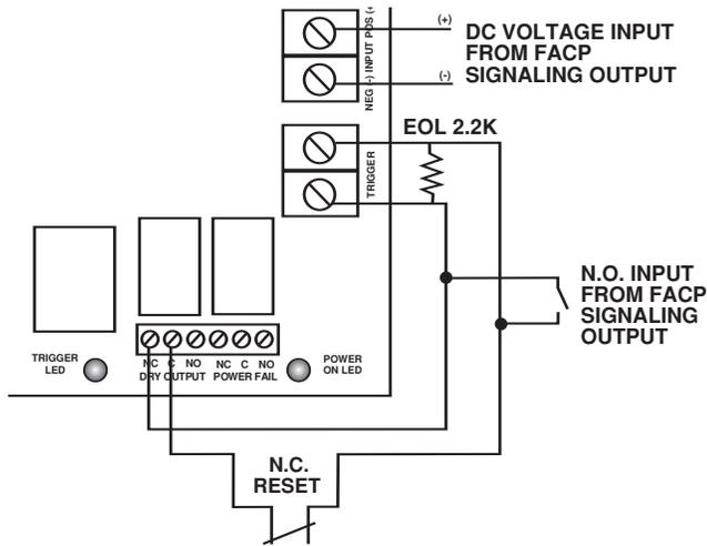
MOM5 module shown with with wet and/or dry normally open fire alarm trigger inputs (**Latching with Manual Reset**):
