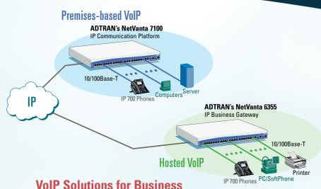
ADTRAN offers a wide range of attractive VoIP solutions for today's market. ADTRAN IP phones can be used with the NetVanta 6355 IP Business Gateway for hosted applications, or with the NetVanta 7000 Series for premises-based VoIP applications.
