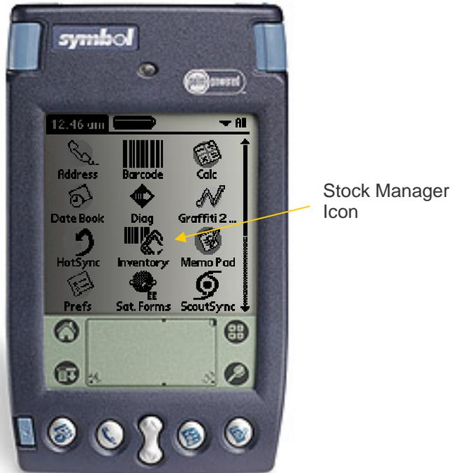
**Figure a.** Symbol SPT 1550 Barcode Scanner
