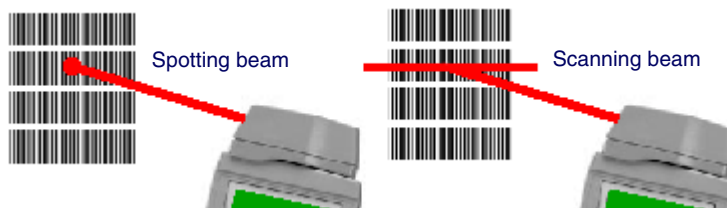
Figure 21: Falcon 31x/32x/34x Long-Range Laser Operation
