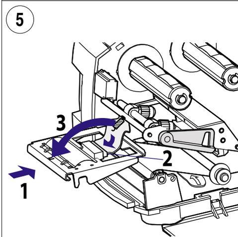
Slide in the new printhead (1), connect the printhead cable (2), and hook the spring into position (3.)
