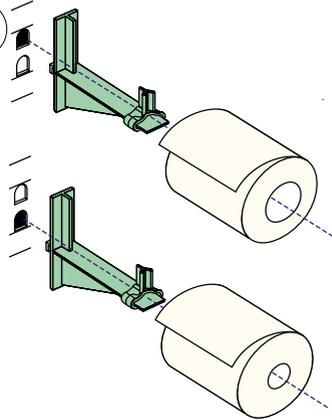
Check that the media supply roll post is in the correct position for the size of the media roll. The post is easier to move if first rotated  $\frac{1}{4}$  of a turn. Push the new roll as far in as it will go and adjust the edge guide.
