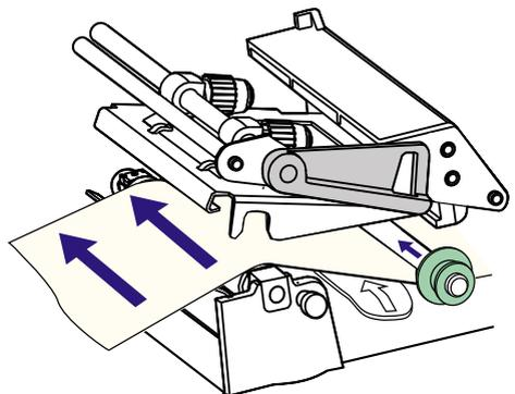
Push the media as far in as it will go and adjust the edge guide ring according to the width of the media.
