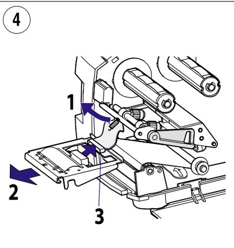
Unhook the spring (1), pull the printhead forward (2), and disconnect the cable (3.)
