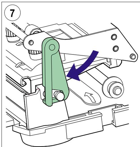
Turn the printhead lift lever clockwise to engage the printhead.
