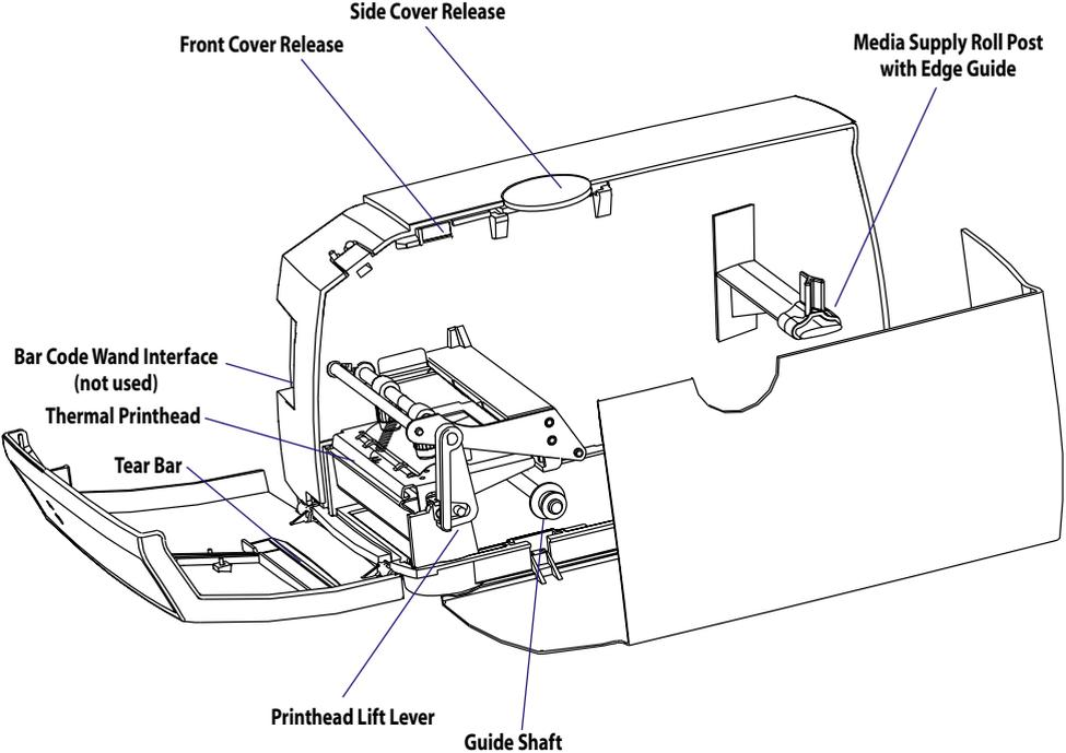
*The left side of the case is not designed to be opened by the operator.*
