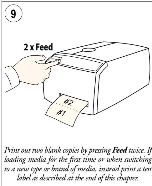
Print out two blank copies by pressing **Feed** twice. If loading media for the first time or when switching to a new type or brand of media, instead print a test label as described at the end of this chapter.
