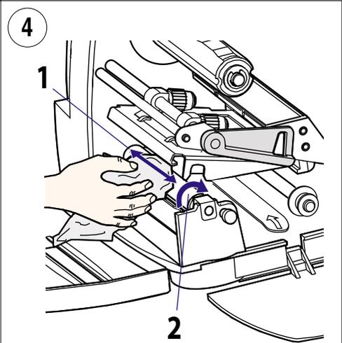
Clean the exposed face of the platen roller while rotating it manually.
