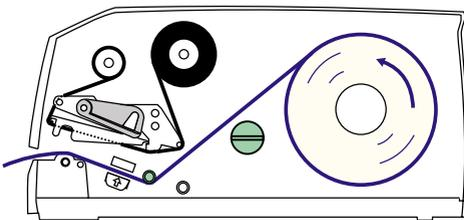
Route the media between the guide rollers, between the two parts of the ribbon/media sensor, over the platen roller, and out through the feed-out slot.
