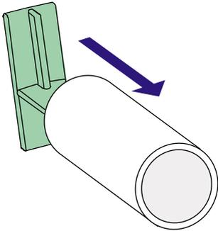
Remove any empty core from the media supply roll post. It is not necessary to remove the edge guide.
