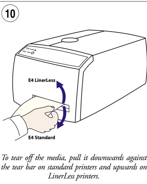
To tear off the media, pull it downwards against the tear bar on standard printers and upwards on LinerLess printers.
