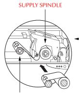
**3.** Load ribbon onto the supply spindle (under print head carriage) and empty core (with tape attached) onto the take-up spindle. Make sure the ribbon comes off of the top of the supply spindle and feeds to the top of the take-up spindle.
