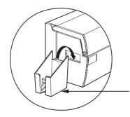
Install Card Output Hopper onto printer by hooking over button edge of card exit aperture.
