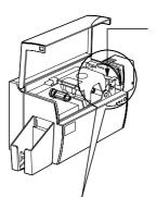
**2.** Open Printer cover and remove the yellow reminder tape from the location for the Cleaning Cartridge.
