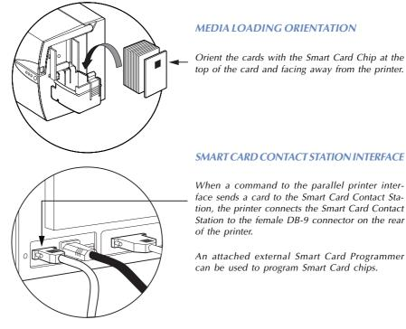
Orient the cards with the Smart Card Chip at the top of the card and facing away from the printer.
