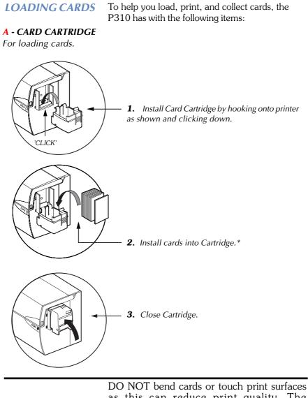
DO NOT bend cards or touch print surfaces as this can reduce print quality. The surface of the cards must remain clean and dust free. Always store cards in an enclosed container. Ideally, use cards as soon as possible. If cards stick together, carefully shuffle them.
