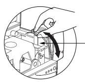
Open Cover, and adjust lever to correct position. Repeat for different card thickness. (Factory setting is for 30mil (0.762mm) card thickness. See diagram below:
