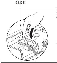
**4.** Push down on the Print Head Lock Lever until an audible 'click' signals the locked-down position.
