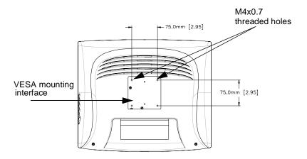
NOTE: The above drawing displays the VESA mounting interface after the removal of the mounting cover and base.
