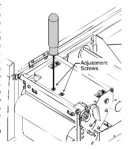
☑ Note: Excessive pressure can reduce the service life of the printhead and platen roller. Contact Datamax Technical Support with any questions regarding this procedure.
