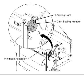
Whenever using labels of a different width, readjust the Leveling Cam.
