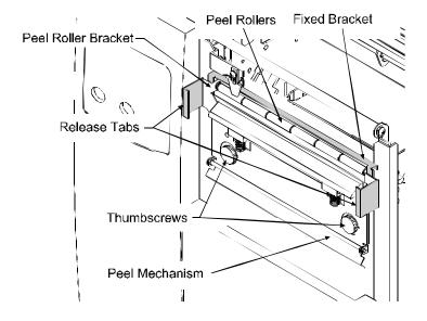
• Thread the media over the top of the Fixed Bracket, behind and under the Peel Roller Bracket, then down to the Media Rewind Hub.
