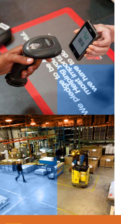
You can also read codes that are damaged or poorly printed, which is something that laser scanners would never be able to. Imagers have a greater tolerance when the print isn't quite dark enough or faded since they are processing images instead of reflected light. In the case of damaged codes, if there isn't a clean straight line across the code a laser can't read it. An imager is **smart** enough to still extract the information from the code as long as it can be read somewhere in it.
